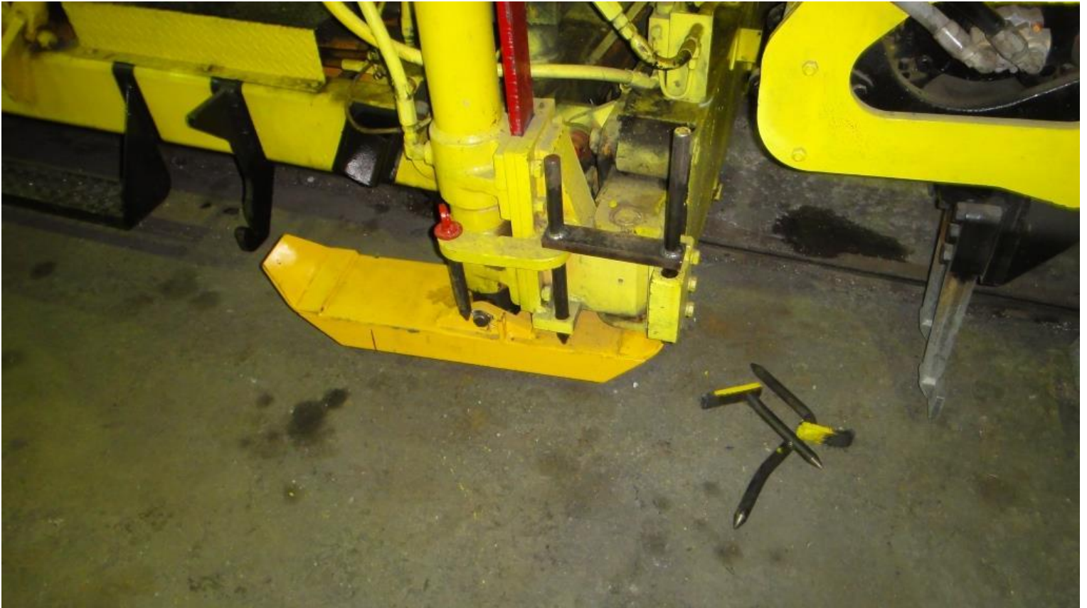
Cliff made new keeper pins for the jacking system on the tamper
